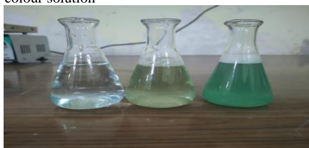
Fig 1: a) CuSO 4 solution; b) CuSO 4 and plant extract; c) CuO formed nanoparticles
